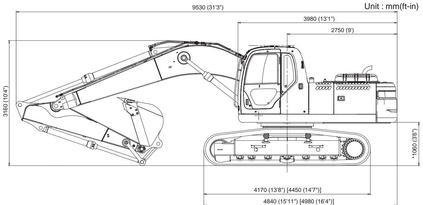
2.2.3 E215B/E215BLC [5.65m (18ft-6in) Boom+3.5m (11ft-6in) Long Arm+0.70m<sup>3</sup> (0.92cu•yd) Bucket Shoe]
