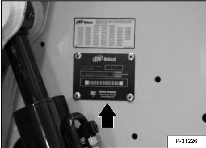
The loader serial number plate is located on the outside of the loader frame [Figure 2].
