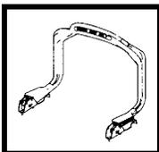
5. Check lift arm support device, replace if damaged.
