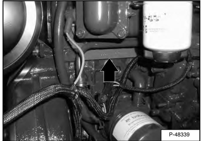
The engine serial number is located on the engine block [Figure 3].
