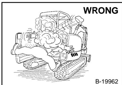
⚠ Stop, cool and clean engine of flammable materials before checking fluids.
