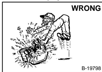
⚠ Lead-acid batteries produce flammable and explosive gases.
