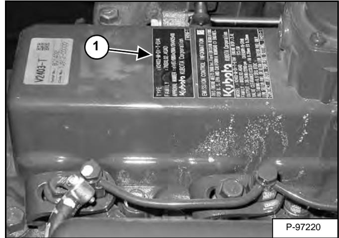
The engine serial number (Item 1) [Figure 3] is located on the top cover.
