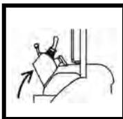
22. Inspect the X-Change™ for wear or damage. Repair or replace damaged parts.
