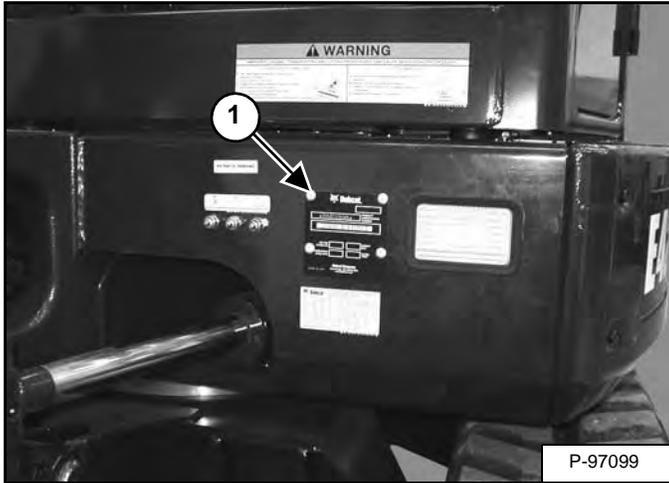
The excavator serial number plate (Item 1) is located on the frame of the machine in the location shown [Figure 1].
