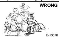
Stop, cool and clean engine of materials flammable before checking fluids.
