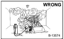
good ventilation Have when welding or grinding painted parts.
