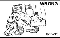
Disconnecting or loosening any hydraulic tubeline, hose, fitting, component or a part failure can cause lift arms to drop. Do not go under lift arms when raised supported unless by approved lift arm support device. Replace it if damaged.
