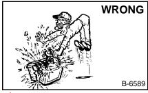
Lead-acid batteries produce flammable and explosive gases.
