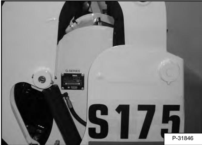
The loader serial number plate is located on the outside of the loader frame [Figure 1].
