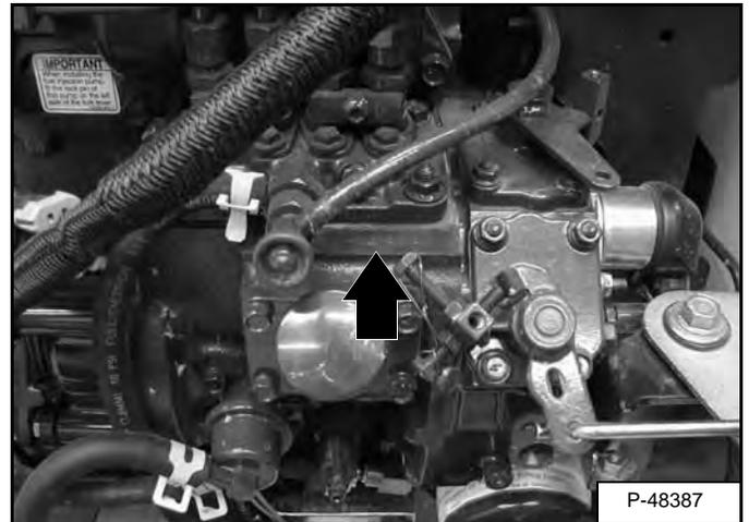
The engine serial number is in the location shown [Figure 2].
