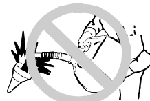
NO STATIC ELECTRIC DISCHARGE
