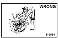
Lead-acid batteries produce flammable and explosive gases.
