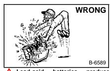
Lead-acid batteries produce flammable and explosive gases.
