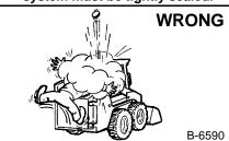
A Stop, cool and clean engine of flammable materials before checking fluids.
