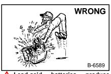
Lead-acid batteries produce flammable and explosive gases.
