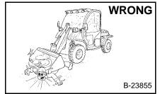
Disconnecting or loosening any hydraulic tubeline, hose, fitting, component or a part failure can cause lift arm or implement to drop. Do not go under lift arm when raised unless supported by an approved lift arm support device or under raised implement without proper supported. Replace if damaged.
