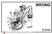
Lead-acid batteries produce flammable and explosive gases.
