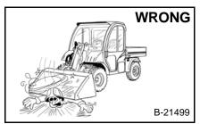
Disconnecting or loosening any hydraulic tubeline, hose, fitting, component or a part failure can cause lift arm or cargo box to drop. Do not go under lift arm or cargo box when raised unless supported by an approved lift arm or cargo box support device. Replace it if damaged.
