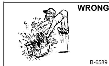
Lead-acid batteries produce flammable and explosive gases.
