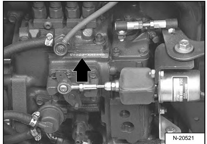
The engine serial number is in the location shown [Figure 3].
