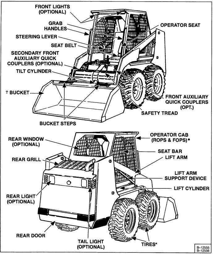
\* TIRES – Flotation tires (optional) are shown. The Bobcat loader is factory equipped with standard tires. + BUCKET – Several different buckets and other attachments are available for the Bobcat loader.
