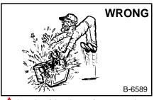
Lead-acid batteries produce flammable and explosive gases.
