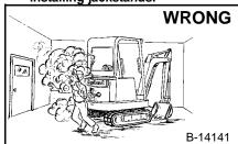
Vent exhaust to outside when engine must be run for service.
