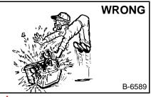
Lead-acid batteries produce flammable and explosive gases.
