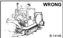
Stop, cool and clean engine of flammable materials before checking fluids.
