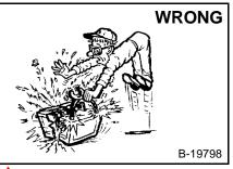
Lead-acid batteries produce flammable and explosive gases.
