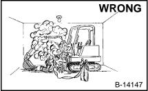
good Have ventilation when welding or grinding painted
