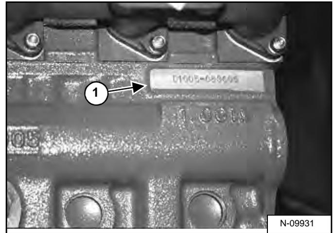
The engine serial number (Item 1) [Figure 3] is in the location shown.
